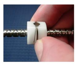
To remove the coil spring that is wrapped around the traveler, locate the end of the spring that is nearest to the small gear. With your fingernail gently lift and push the end of the spring until it is off the traveler. Guide the rest of the spring with your finger while turning the traveler so as to unscrew the spring from the traveler.
