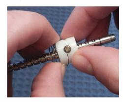
Pull the end of the coil spring over the traveler and by guiding it with your finger, working a little at a time, slip the rest of the spring into place in the groove.
