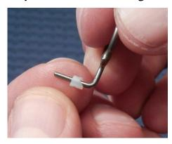
You will notice that the "Quiet-Glide" bushing has a 45 degree cut on one end of it. Place the bushing on the eyelet foot with this end first.
