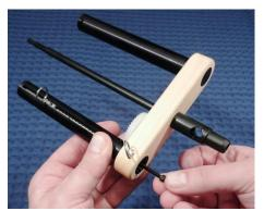
Hold the large gear to keep it from moving and install the handle screw into the threaded hole in the end of the travel screw.
