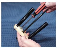
Replace the large gear. If your model has a gear with a bevel on one side of the center hole, the bevel must face out (away from the flier base). Install the gear screw and tighten it with a household screwdriver.
