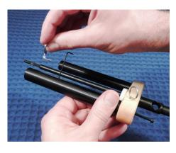
Remove the eyelet by sliding it away from the base of the flier. Make sure the little white "Quiet-Glide" bushing does not fall into the travel arm.
