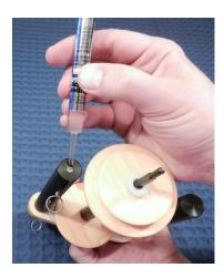
On each end of the flyer shaft where the bobbin gears ride on the shaft, a light application of any grease or Vaseline should ensure that the bobbin winds freely and without noise. You can use oil here as well; however, the grease is better at preventing any bobbin knocking noise.
