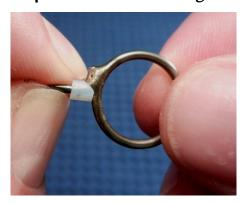
Push the bushing up over the 90 degree turn in the eyelet foot and up against the eyelet. Make sure that the cut in the bushing is situated so that it meets the point at which the eyelet foot is soldered to the eyelet itself.
