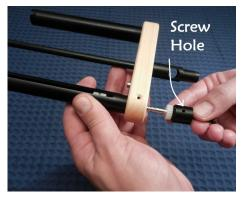
Slide the travel screw assembly back into the flier arm. Be sure to align the screw hole in the top of the end bearing with the hole in the top of the flier base before pushing it in completely.
