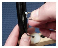
Holding the flyer at a 90 degree angle to the floor will help the bushing to stay in place as you insert the arm of the eyelet back into the small hole on the side of the white traveler.
