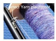
If your yarn should suddenly fail to wind onto the bobbin, first check the yarn to make sure it hasn't flipped itself around the moving eyelet. This occurs occasionally when all tension is released on the
