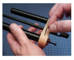
Use the Allen wrench from the tool kit to verify that the hole in the end bearing is lined up with the hole in the flyer base. Insert the Allen wrench into the eyelet hole and move the Allen wrench in a circle. The Allen wrench should go through both parts which will ensure that the two parts are properly aligned for the next step.
