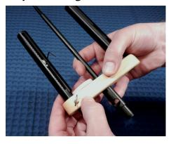
Turn the large gear until the set screw for the moving eyelet is visible. Insert the Allen wrench and loosen the screw 1 to 1½ turns. Leave the Allen wrench in place.
