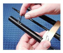
Use the Allen wrench again to tighten the set screw so that it will hold the eyelet in place. Don't over tighten it -- just snug will do fine.
