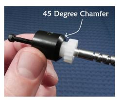
The black front bearing has one end that has a sharp edge and the other side has a 45 degree chamfer cut into it. Slip the front bearing over the hub of the small gear with the 45 degree chamfered end toward the gear teeth.
