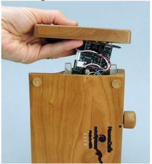
4. Pull the circuit board out of the base and unplug the tachometer sensor, then set the face aside.
