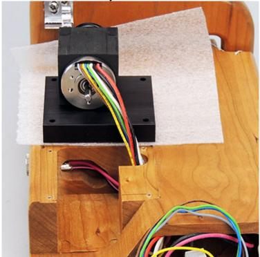
8. Pull back the EPDM rubber cushion, then use a short piece of tape to attach the bare end of the grounding wire to the motor. The wire's insulation is flush with the end of the motor (arrow).
