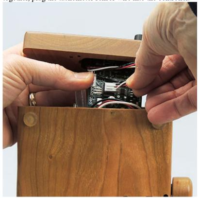
17. Hold the controller and the face together as you slide the controller all the way into the base. Be careful to line up the alignment pins and the polyurethane rods that hold the controller board and face in place as you do this. Carefully tighten the 3 screws holding on the face, as you ensure that no wiring is caught between the face and the base at the seam where they come together. Do NOT force things together!
