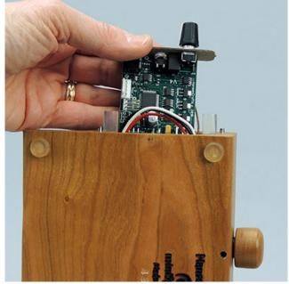
16. Insert the front panel of the controller board into the pocket of the miniSpinner's face piece, making certain the wiring for the tachometer sensor remains in its channel. While holding these together, plug the tachometer sensor wire into the controller.
