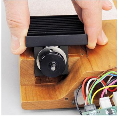
7. Use the pad to protect your miniSpinner from being scratched by the heat sink as you rotate the heat sink/motor assembly to the rear so it sits on the heat sink, upside down.
