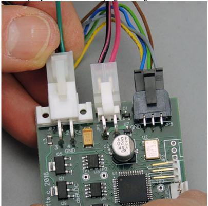
15. Arrange the motor wires on the top and bottom of the controller board and place the board halfway into its pocket. Try to arrange the wiring as you do this so it's not all jammed behind the circuit board at the bottom of the pocket. **Note the controller board is "upside down!"**
