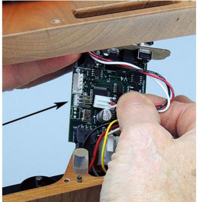
5. Set your miniSpinner upright and use a #1 Phillips screwdriver to unscrew the four screws holding the heatsink in place.
