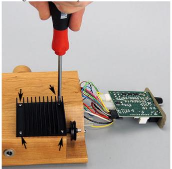
6. Pull up on the heat sink/motor assembly to remove it from the base. The motor is attached to the heat sink with thermally conductive tape and sits in an EPDM rubber cushion, which is a tight fit in the base.
