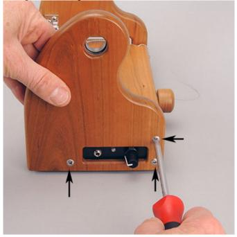
3. Set your miniSpinner on its "back" and gently remove the face. There are two locating pins that hold it in alignment with the base, so it may require you to rock it slightly as you pull to separate it from the base. Note: The face is connected to the controller board by the tachometer sensor wiring.
