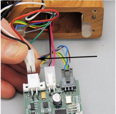
13. There is an unused position in the motor plug housing. The jumper wire goes into this hole.
