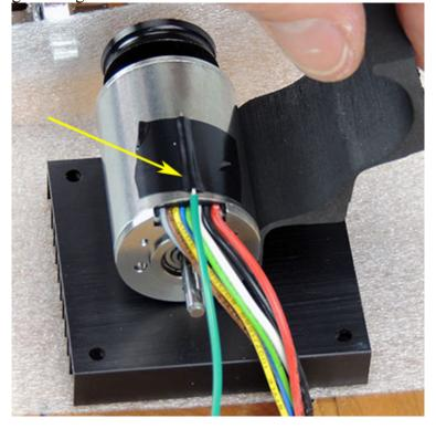
9. Pull the circuit board completely out of the pocket in the base, then thread the other end of the jumper wire into the circuit board pocket so that it sticks out the front (arrows).
