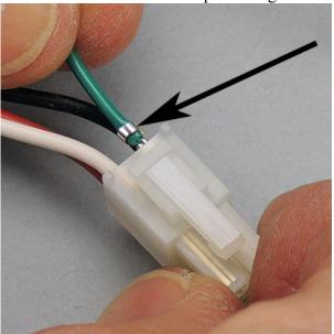
14. Plug the motor back into the controller board, making certain the plug latches into place, and that the pin you inserted in the plug for the green wire remains in place in the plug housing.
