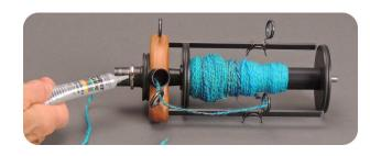
Note: You may need to adjust the latch for the correct endplay of about 1/16" (1mm) between the bobbin end and the rear spherical bearing. Slightly loosen the screws holding the latch to the base of your miniSpinner, slide it to get the correct amount of endplay, then tighten the screws. See <a href="http://hansencrafts.com/repairs/for detailed instructions">http://hansencrafts.com/repairs/for detailed instructions</a>.
