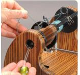
Prepare the bobbin for spinning by threading its leader through the moving eyelet on the right side of the flyer arm, through the right-hand stationary eyelet at the front of the flyer, then use the orifice threader to pull the leader through the flyer orifice.
