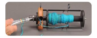
Note: You may need to adjust the latch for the correct endplay of about 1/16" (1mm) between the bobbin end and the rear spherical bearing. Slightly loosen the screws holding the latch to the base of your miniSpinner, slide it to get the correct amount of endplay, then tighten the screws. See http://hansencrafts.com/repairs/for detailed instructions.
